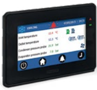
Latest-generation touch screen user terminal.
